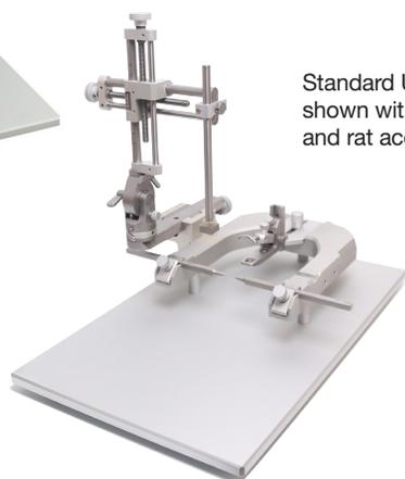
Standard U-Frame Stereotaxic Instrument, shown with a single manipulator arm and rat accessories
