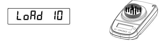
If the number of samples is enough (for example 10 as in figure), then this number will be displayed and it will be possible to go on by loading the pieces to count on the balance pan.
