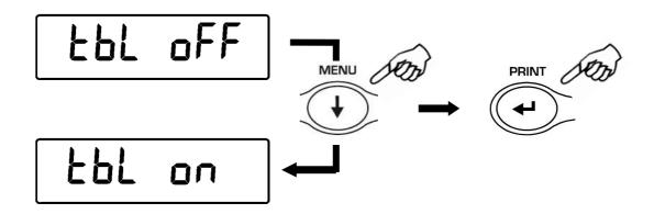
3. After you have choosen the mode **"TBL ON"** the balance will automatically restart and the message **"TABLET**" will appear on the display of balance. <u>From this moment</u> <u>the interface device with the balance is the tablet.</u>
