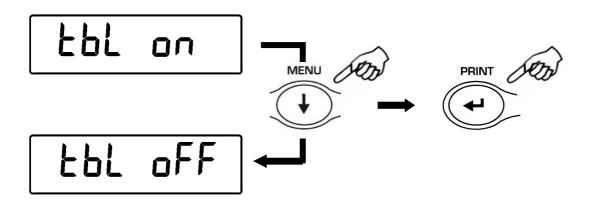
6. After you confirm with the **PRINT** button, the balance will restart automatically and will return to standard working mode.
