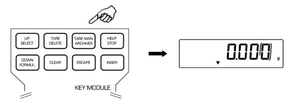
2. Press **CLEAR** to set at zero the previous value (if any) then insert the new value using the alphanumeric buttons placed on the bottom part of alphanumeric keyboard.
