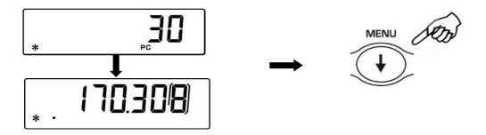
2. In order to display the weight of single piece from the total number of pieces press and keep pressed the **MENU** button until the acoustic alarm gets mute. 3. Press again the **MENU** button to display the number of pieces.
