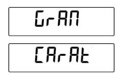
3. Press **PRINT** button to confirm or **MENU** button to shift to the other weight unit.
