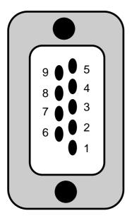
CONNECTOR 1: CONNECTION FOR KEYPAD, PC AND PRINTER
