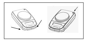
Connect power supply to connector 2 located on the rear panel of the unit (see par. 5).
