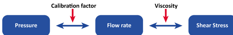
Figure 36 – Influence of the calibration factor and viscosity on the parameters of the PumpControl software.
