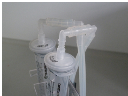
Figure 54 – Cross the tubing on top of the reservoirs to test if the problem is with the Perfusion Set or in the valve block (valve 1).
