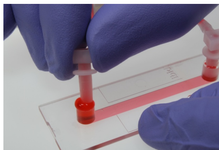
Figure 33 – Connect the second Luer adapter to the \mu -Slide.
