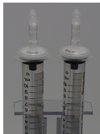
Figure 27 – Connect the filters of the Perfusion Set to the Fluidic Unit tubing.
