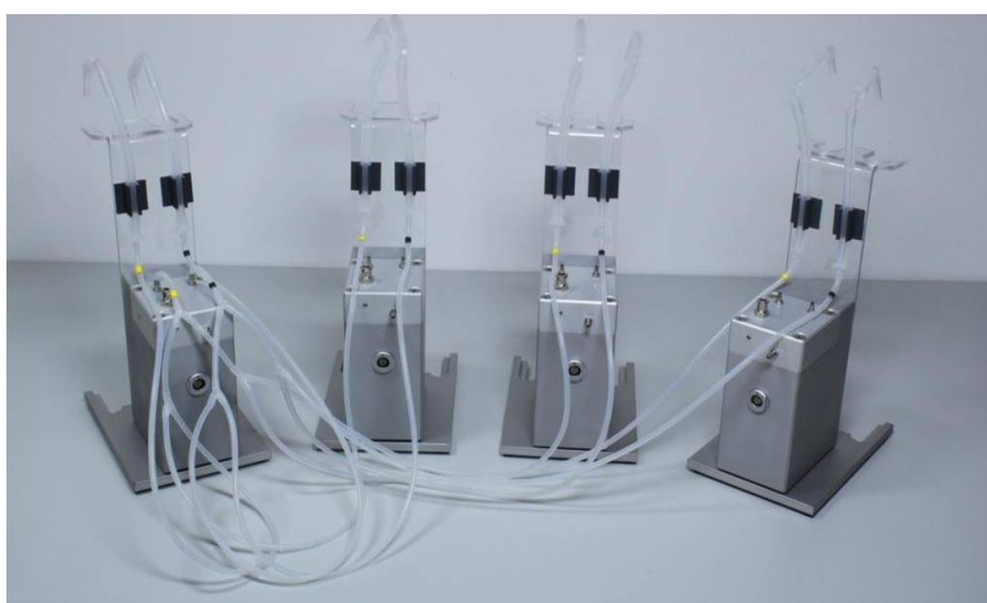
Figure 44 – Oscillatory flow setup with four Fluidic Units (one master and three slaves).
