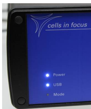
Figure 13 – LEDs on the pump’s front panel indicating the connected USB and power supply.
