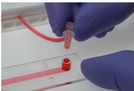
Figure 32 – Fill the reservoir before connecting the Luer adapter.
