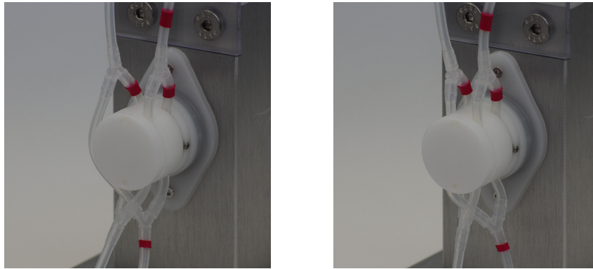
Figure 24 – Insert the tubing coming from reservoir A into the left side slots. The marked tubing goes in the rear slot.
