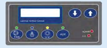
Digital control board with LCD display\* including:
