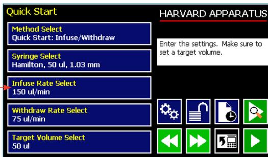
2. Depending on the Method, the appropriate set rate screen will be displayed. To change the units, press the units.
