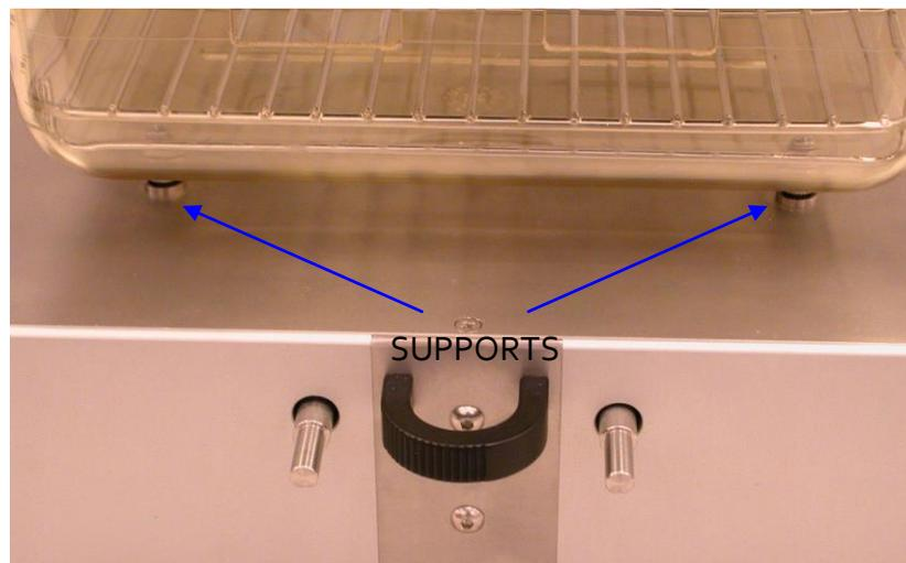
Figure 12: Plastic cage over the supports
