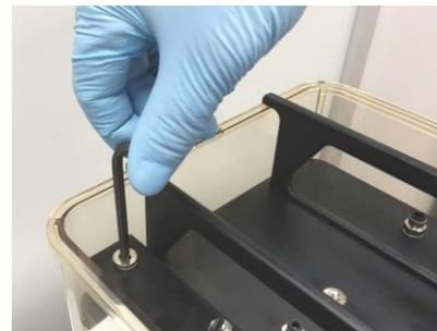
Figure 38: Unscrewing the lid.
