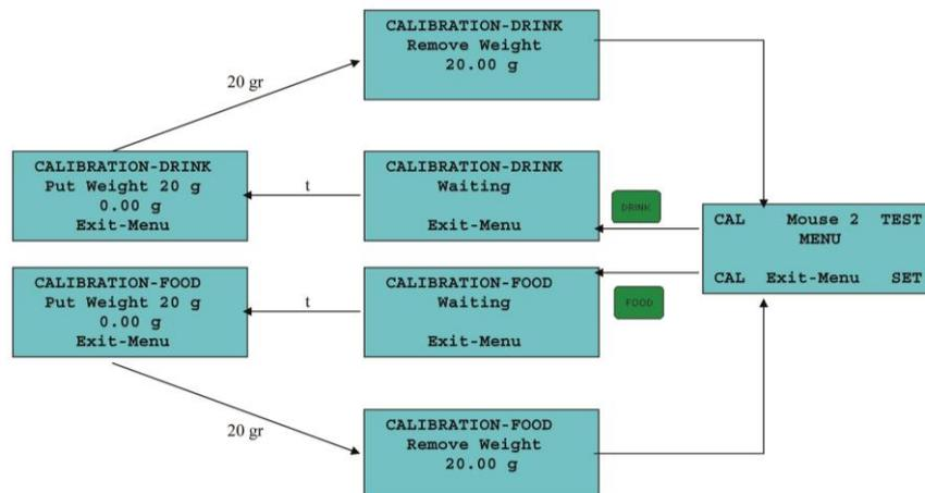
Figure 40: Calibration screen navigation
