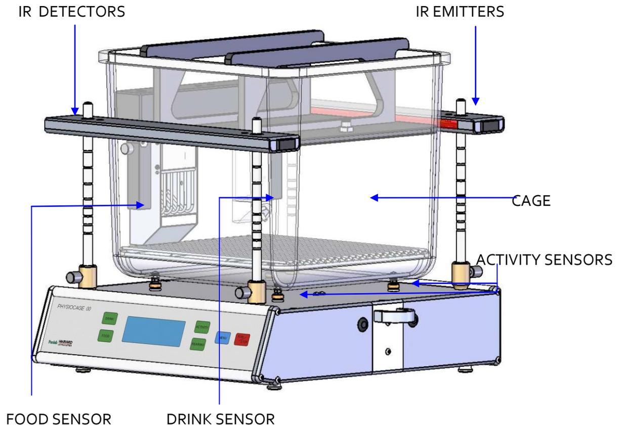
Figure 10: PhysioCage Configuration Components
