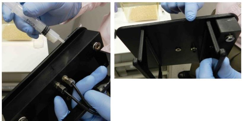
Figure 16: Lubricating the O-ring of the lid
