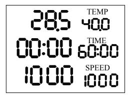
c) Press " peed" or " speed" to set up for the speed. The number will increase or reduce at a rate of 50rpm, release the button when the number reaches exact value, and it will be automatically saved in 3 seconds.
