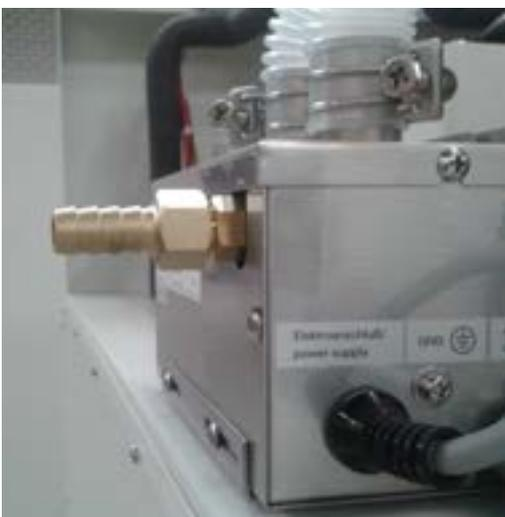
Water inlet for the Ultrasonic humidifier.
